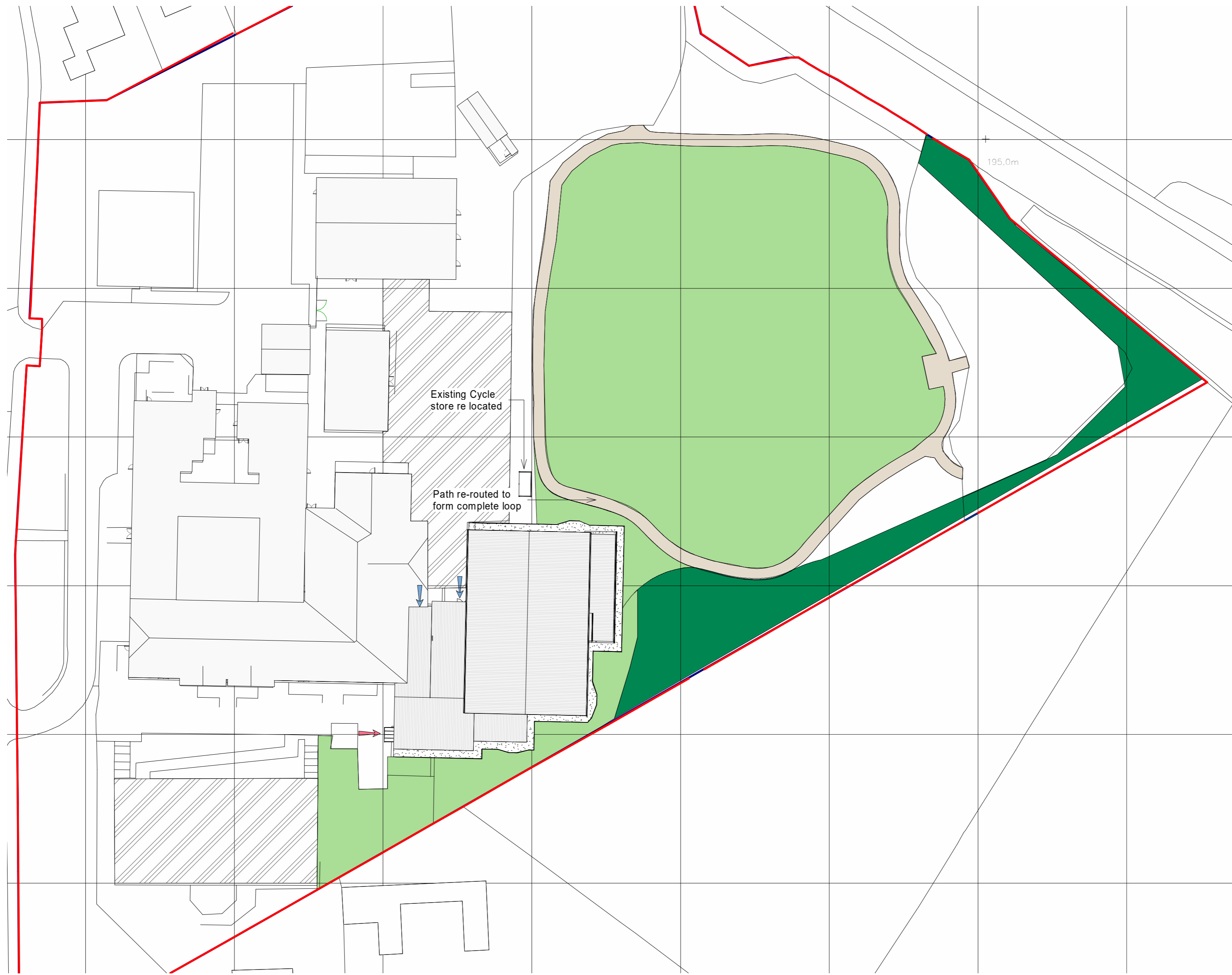
Site Plan - Proposed External Works scale 1:500 @A2
