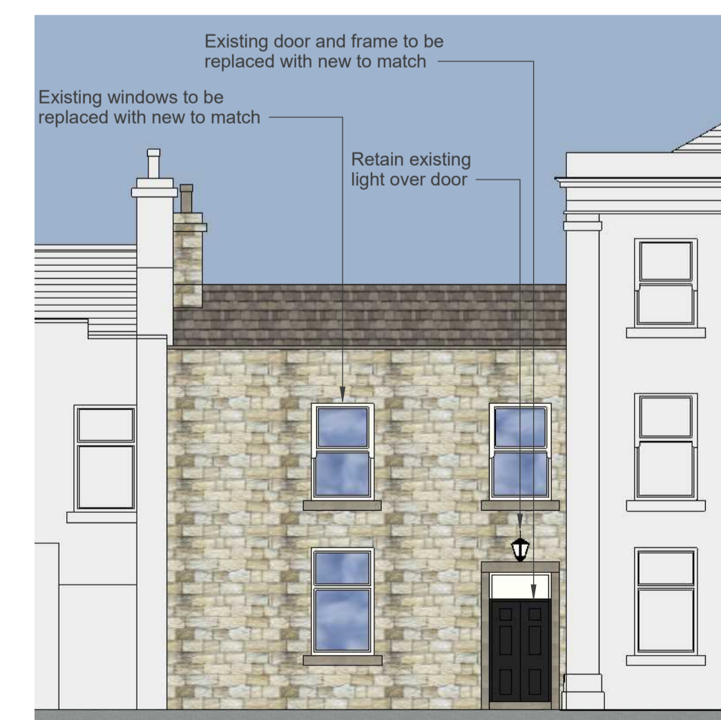
8 Existing West Elevation to Bank St Scale: 1:100
