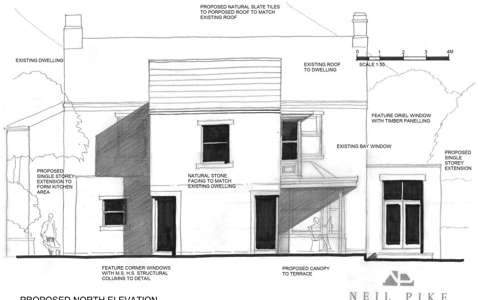
PROPOSED NORTH ELEVATION ALTERATIONS AND EXTENSIONS TO BIRCHCLIFFE, TONACLIFF ROAD, WHITEWORTH IEIL PIKE
