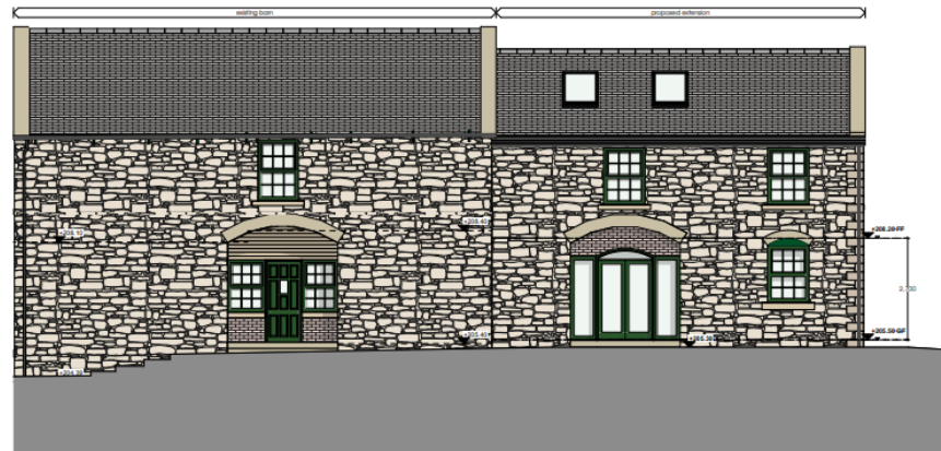
proposed rear elevation (SE) 1:50
