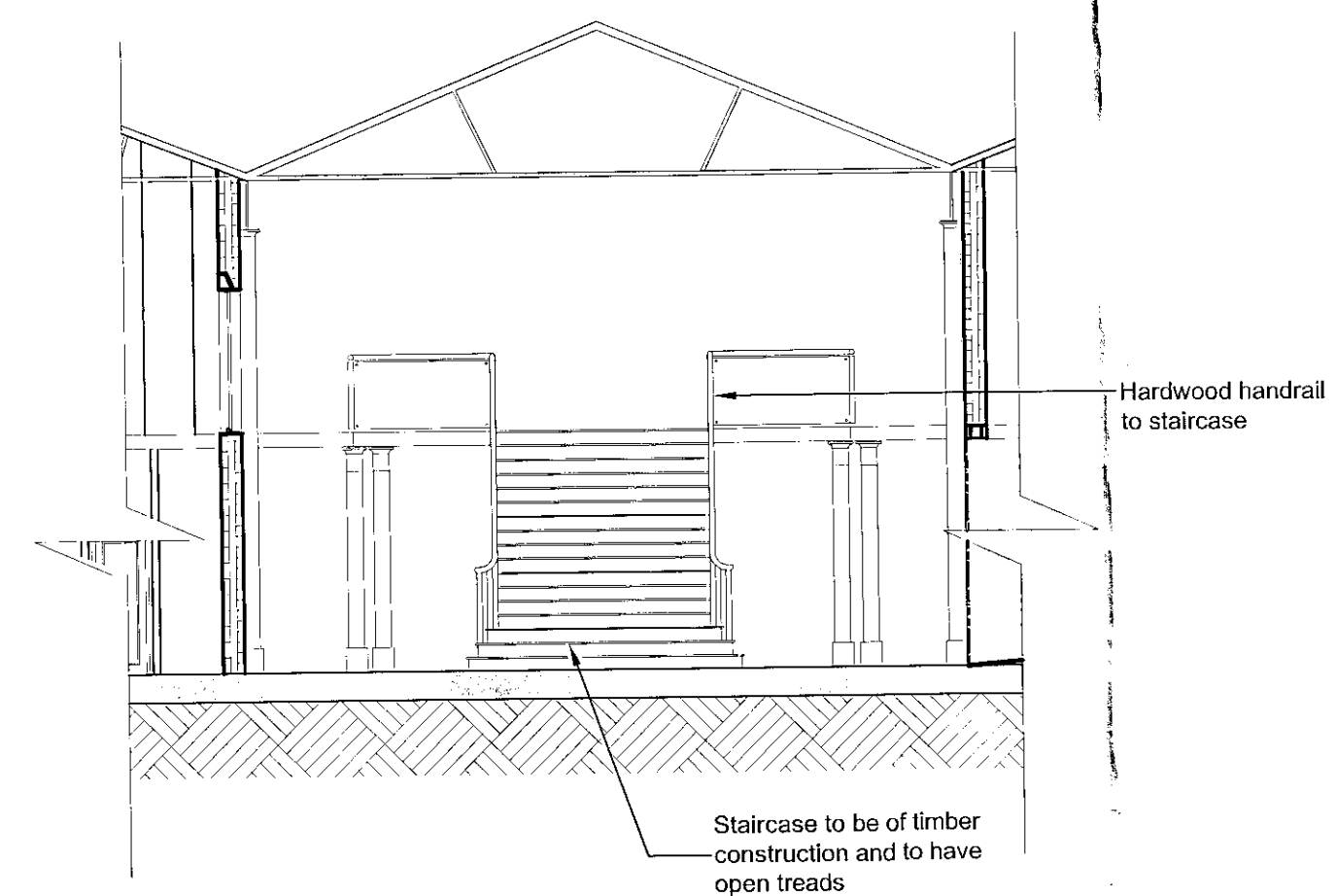
SECTION B - B (STAIRCASE DETAIL)
