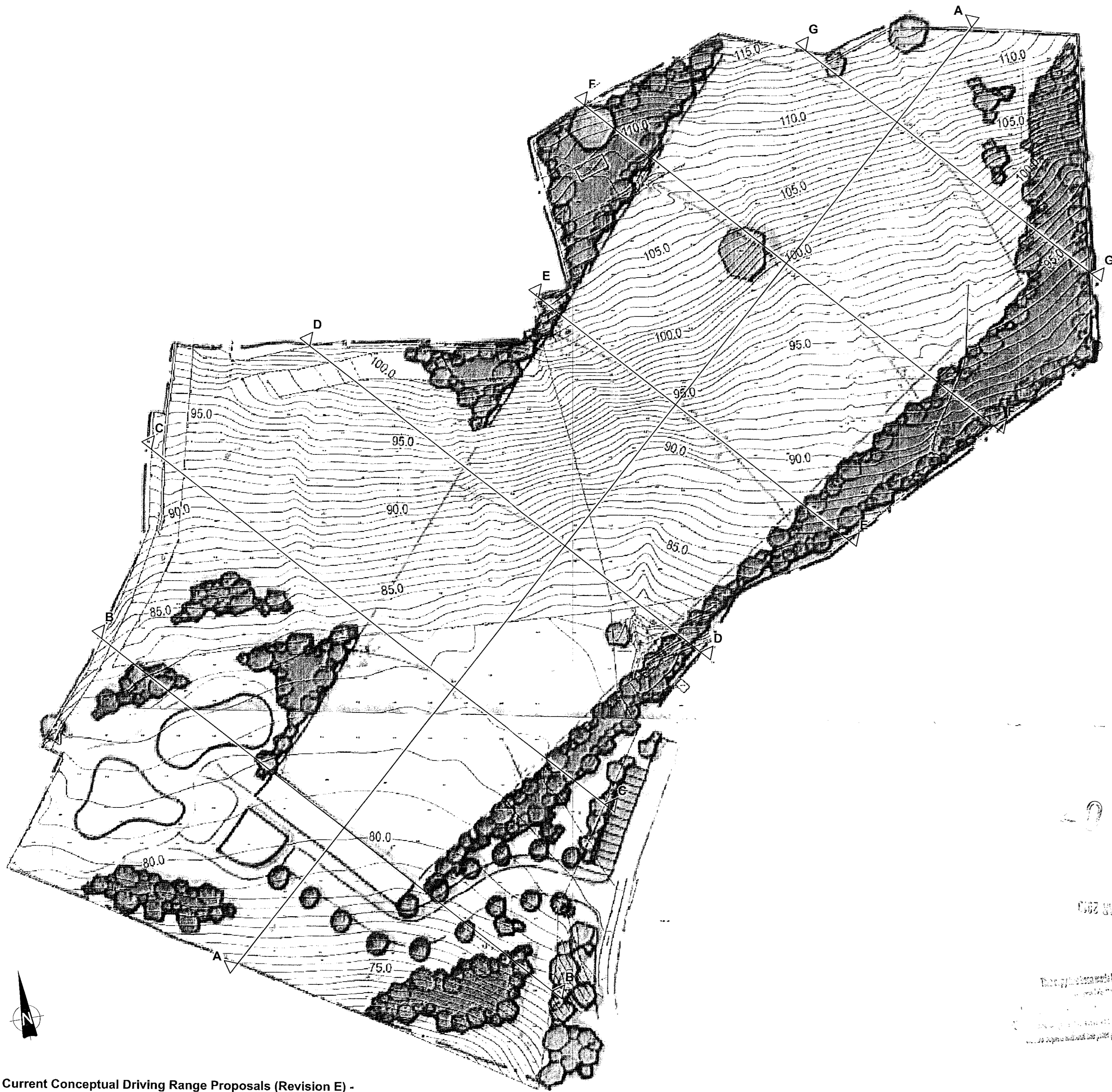
Current Conceptual Driving Range Proposals (Revision E) - Showing Section Line Locations Scale: 1:500
