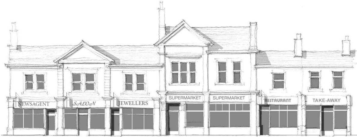
A well designed group of shopfronts with traditional features such as fascias, pilasters and stallrisers integrated into an overall architectural composition.
