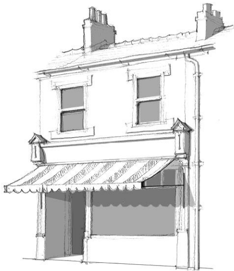
Fabric roller blinds are a traditional feature of the high street. Blind boxes should be located within recessed boxes below the fascia
