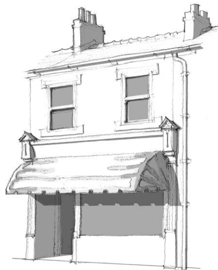
Dutch style canopy blinds are too intrusive and will not normally be acceptable
