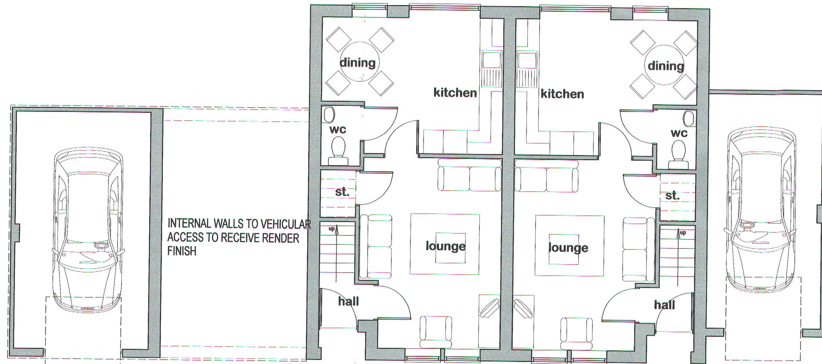
HOUSE TYPE A / PLOTS 5 & 6 PROPOSED GROUND FLOOR PLAN
