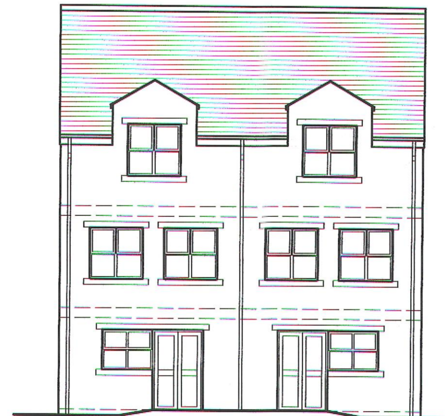
HOUSE TYPE B PLOTS 7/8 9/10 11/12 REAR ELEVATION
