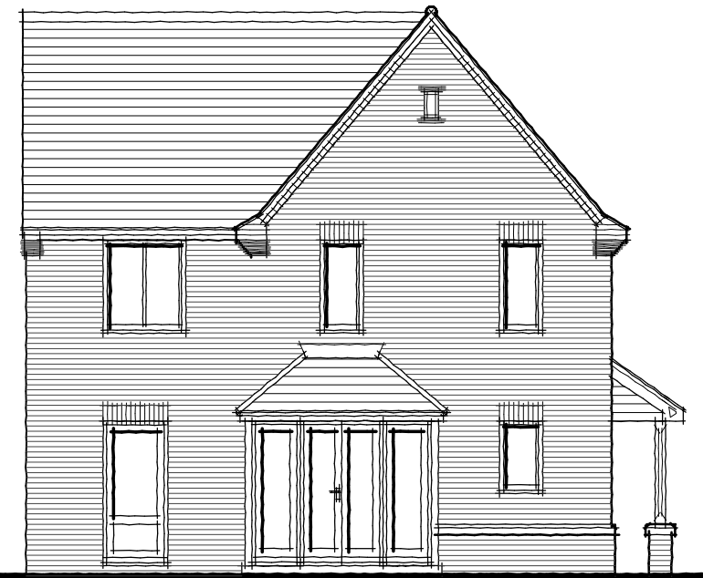
REAR ELEVATION PROJECTING REAR GLAZED BAY & DOORS
