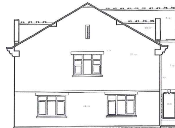
SIDE ELEVATION AS EXISTING (E)
