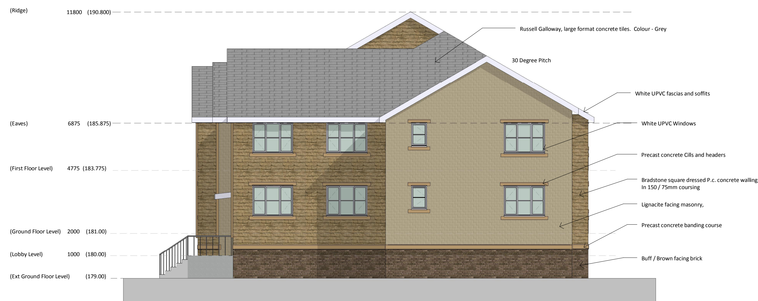
South Facing - Gable Elevation 1 : 100
