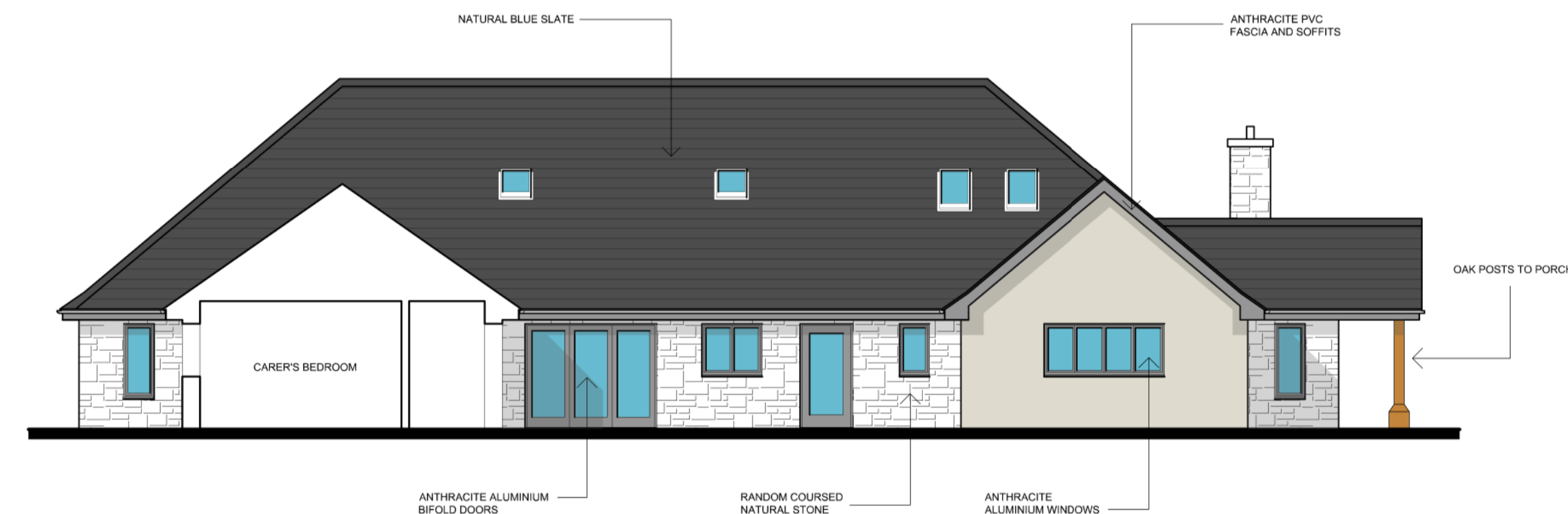
SECTIONAL REAR ELEVATION
