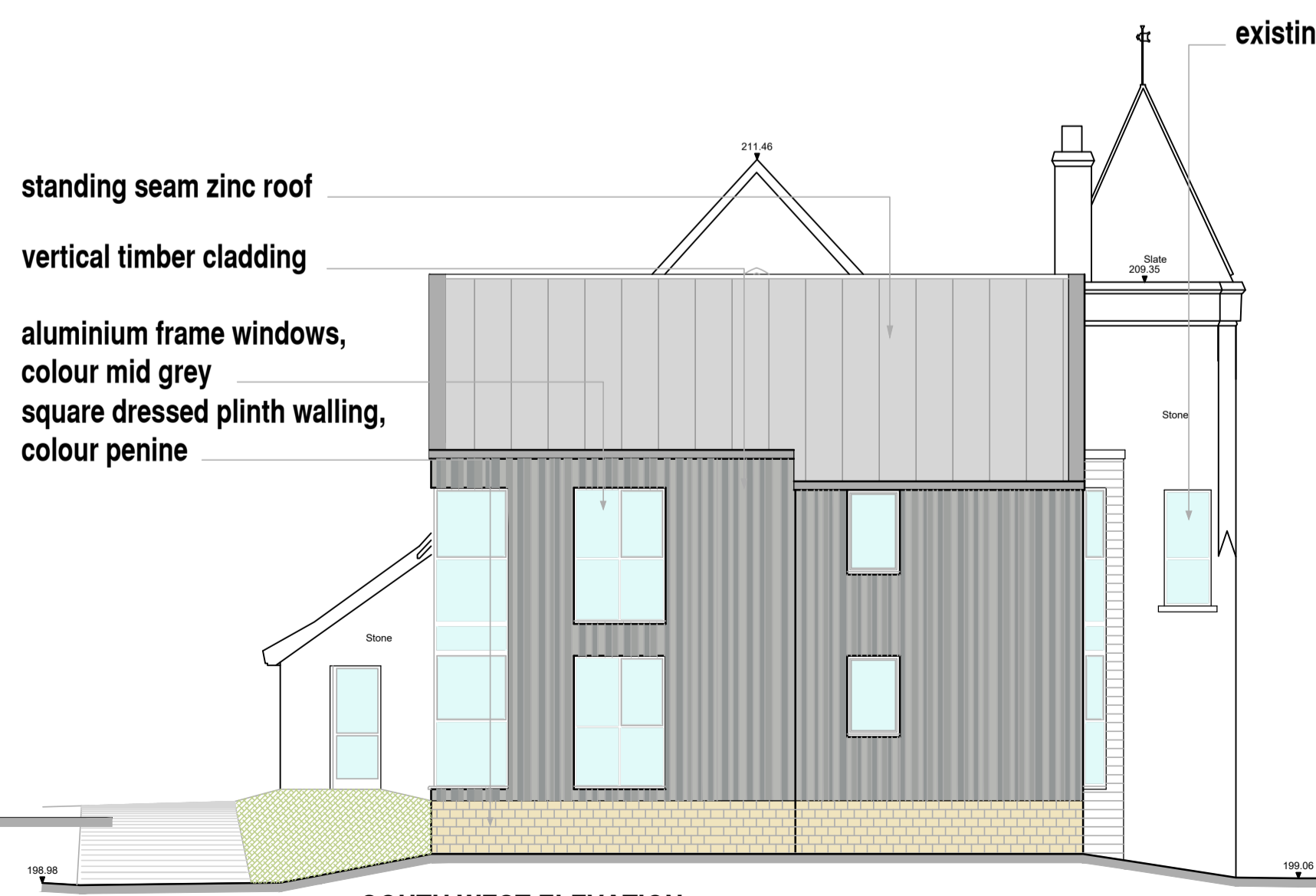
SOUTH WEST ELEVATION
