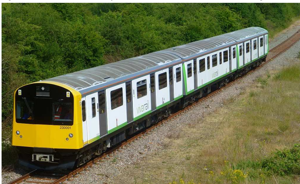
Figure 8: Vivarail Class 230 battery electric train, converted from London Underground stock
