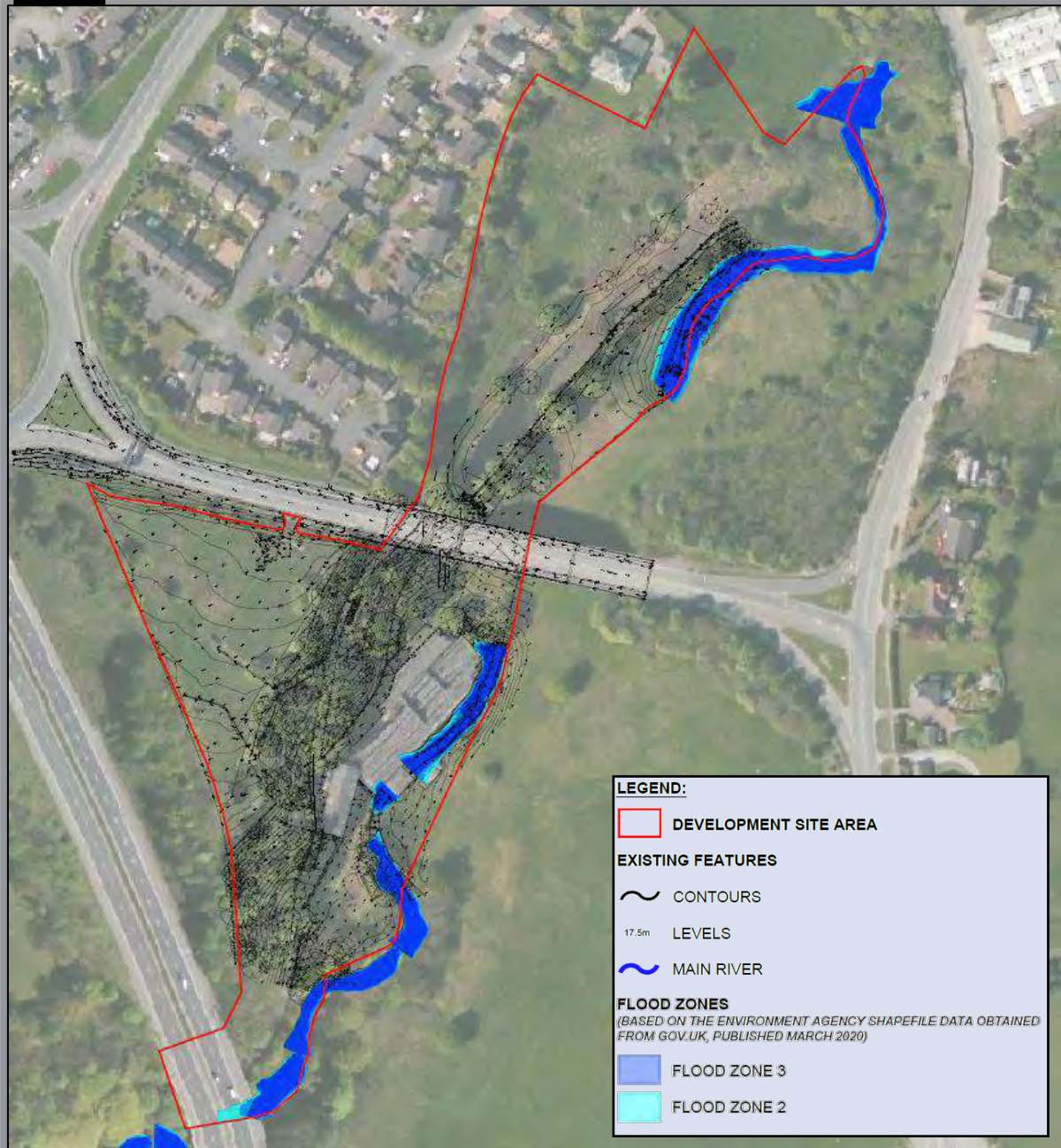
Figure 2: Flood Zone Overlay Plan (Betts Hydro, 2020)
