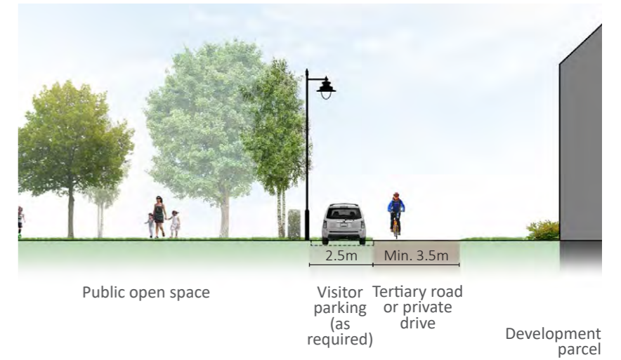
Fig 4.3 Tertiary street cross section
