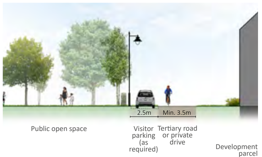
Tertiary street cross section
