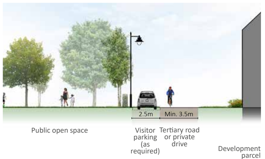
Tertiary street cross section
